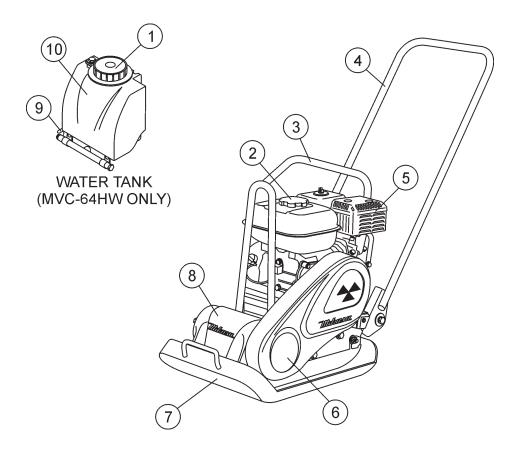
Figure 3. MVC-64H/HW Plate Compactor Components
